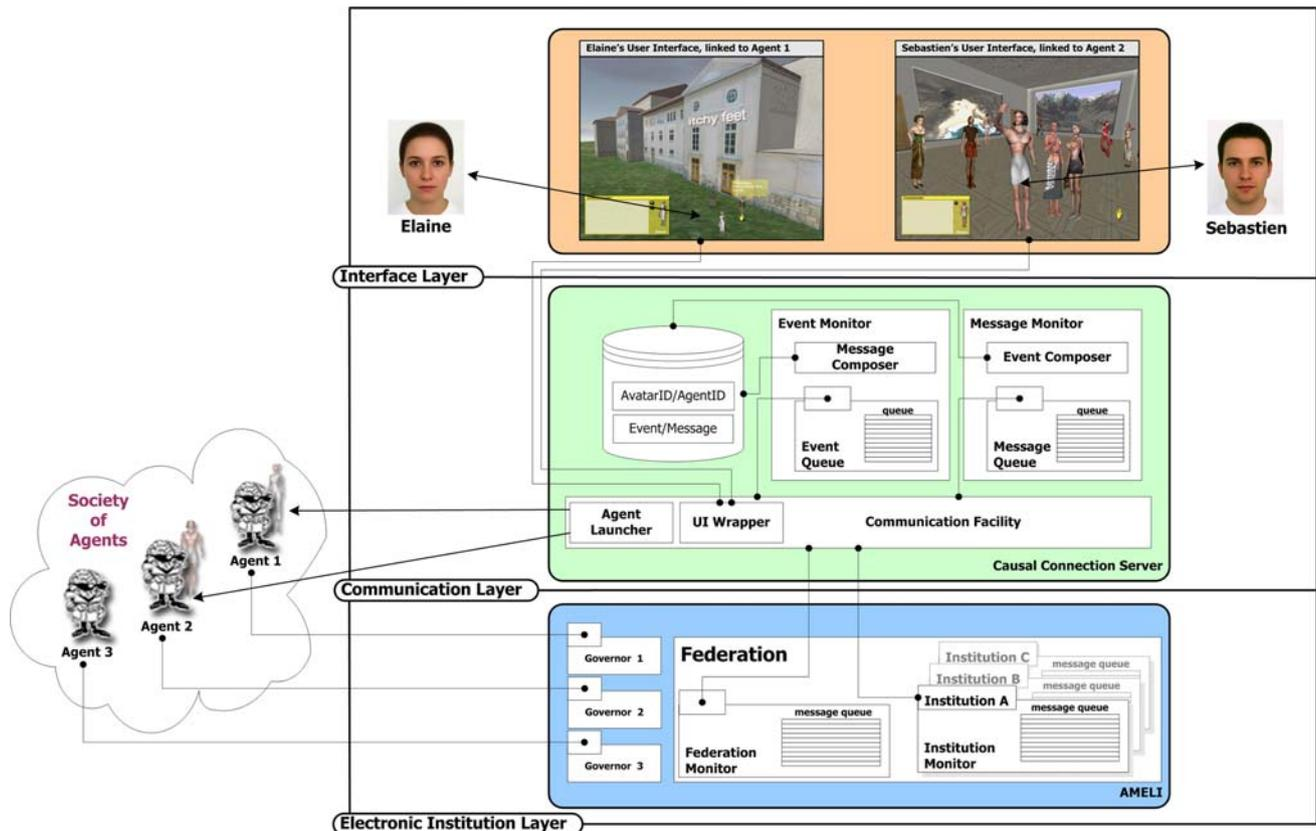
**Fig. 2** The three-layered architecture of 3D Electronic Institutions
